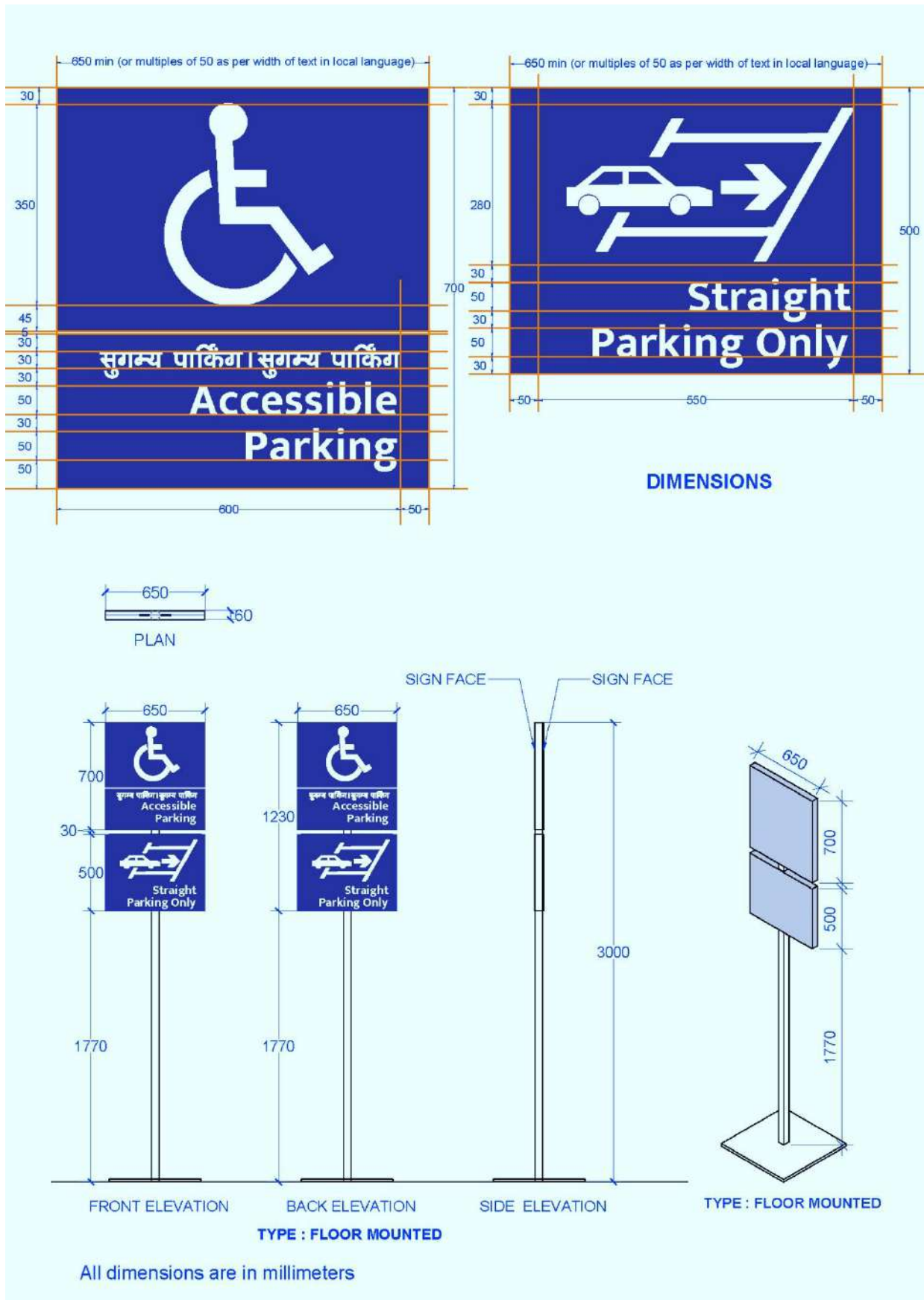
Figure 46: Details of signage for accessible parking
